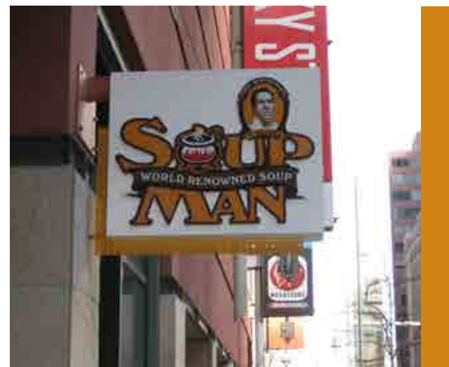
Metal blade sign flag-mounted, letters must be dimensional
