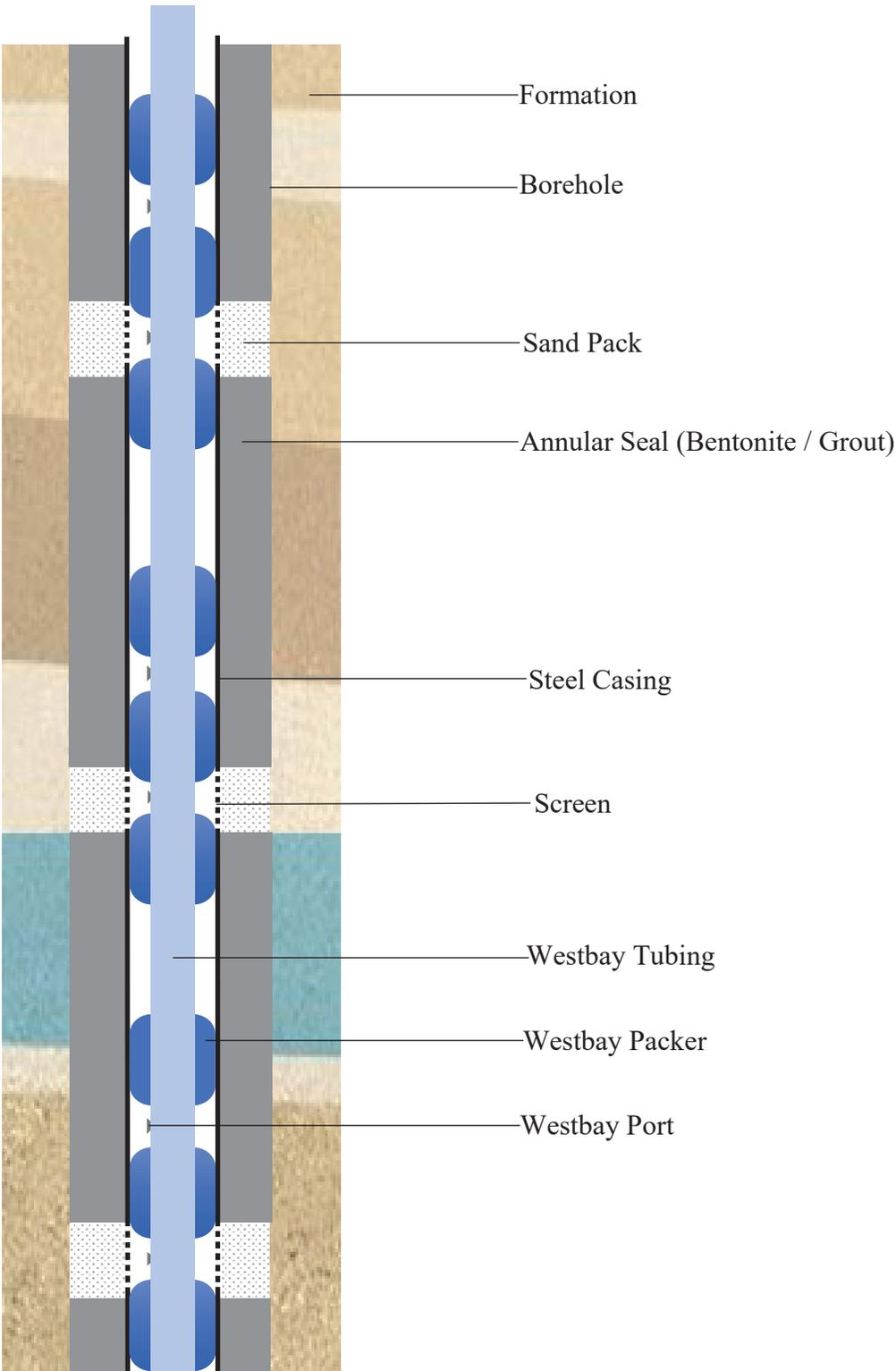
Monitoring Zones      Well Schematic      Schematic Equivalent Depth to Water
